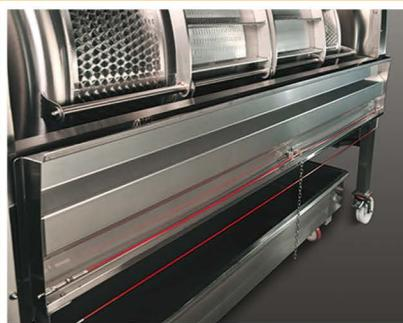
**Upper sides on hinges** open with a handle in the middle. Opening allows easy access to the sliding door, which is particularly helpful when unloading pomace and washing the inside of the cylinder.
