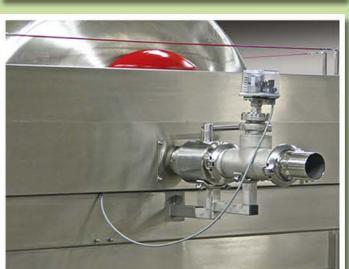
**Level switch** controls the liquid level in the tray. When the minimum and maximum fluid levels are reached, the pump turns on and off or the cylinder rotates with door opening upwards.
