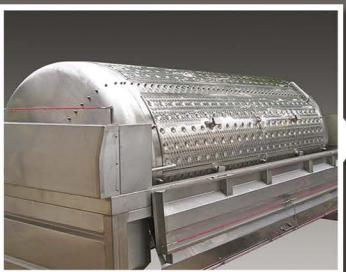
**Cylinder with double coat** is intended for cooling the grapes mass during maceration or pressing. The cooling is possible also during cylinder rotation.
