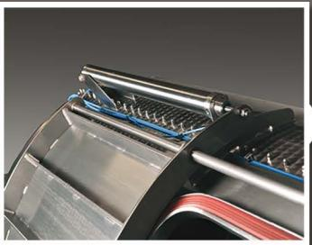
**Sliding doors with pneumatic drive** are operated with a switch on the control panel. The doors can be stopped in any position.
