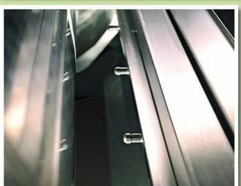
**Cleaning opening on cylinder** allows easier cleaning of the inside of cylinder, because the rinsing liquid drains out constantly.
