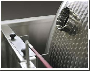
**Central outlet** allows juice to drain from the cylinder through one opening which reduces the effect of oxidation.
