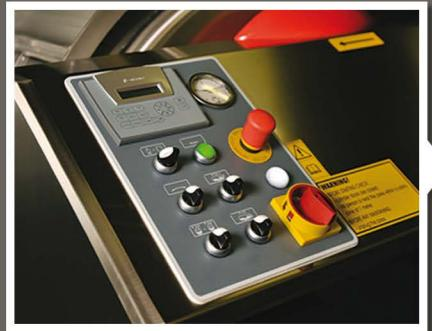
**Automation AE** is part of the standard offer with NIKO VPe presses. The process of grapes pressing is entirely automated with AE automation. The operation is managed on the control panel where the user can monitor the functioning and the current state of the press during the pressing process. The software part includes 8 programs: 4 programs with preset unmodifiable parameters, 2 programs with modifiable parameters, program for axial loading and program for maceration.
