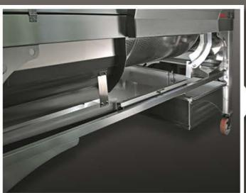
**Alongside sliding tray** consists of several sliding parts. The parts can form a collection tray or can be assembled on the side by pulling them without using great force.
