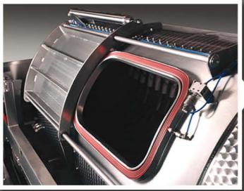
**Watertight sliding doors with inflatable seal.**
