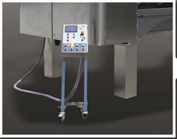
**ALO detached automation:** Control panel can be built-in a detached control box which is connected to the press with a cable.
