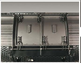
**Non perforated maceration doors** are used when macerating the grapes mass. The doors are non perforated, equipped with a seal and easily installed on the cylinder.
