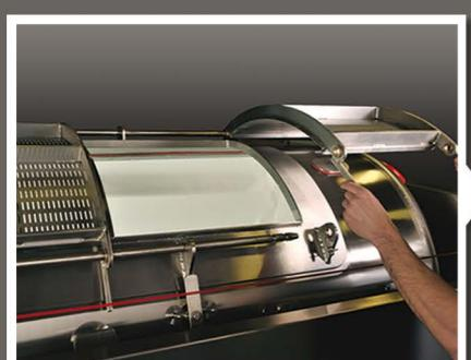
**Axial loading** runs through the axis of the cylinder. The basic version of NIKO VP and HL series includes a manual valve size DN65, DN80, DN100 or DN120.
